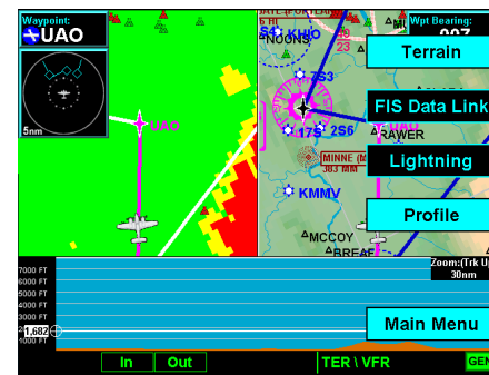
Split Screen showing Custom Map and Flight Plan pages along with the Vertical Profile & Menu Items
